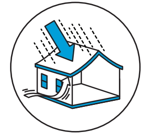
Dynamic Load constantly changing External force that acts through motion such as the wind and rain
